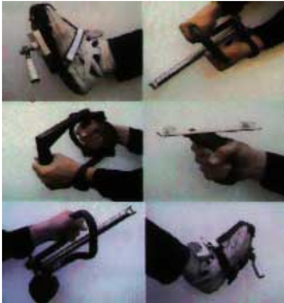
Figure 3: Various couplers can be used as the interface for the machine to rehabilitate or train various sets of muscles.
