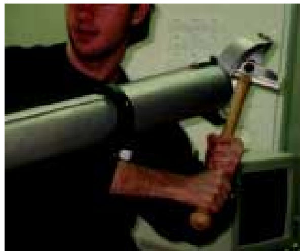
Figure 2: The gimbal handle can be interchanged to activity specific grips such as the baseball handle.
